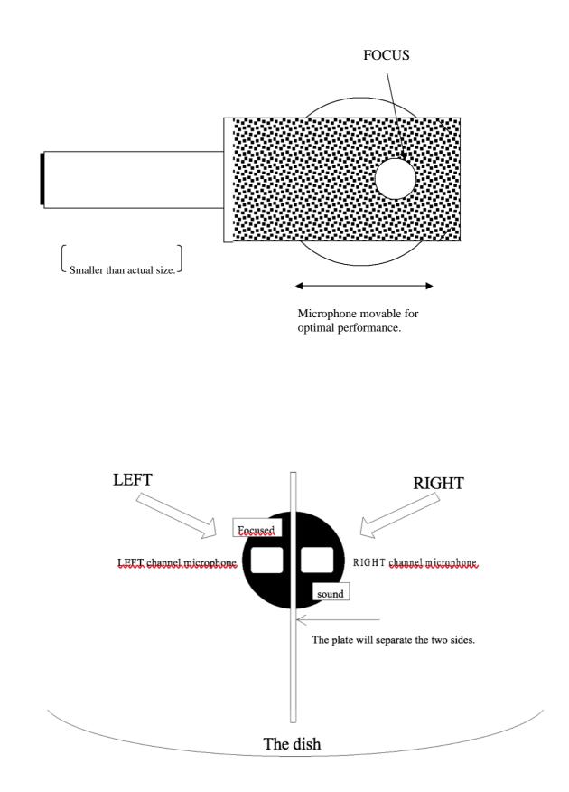
**STEREO MK3:** The plate separates the two sides from each other, while the focused sound will affect the two microphones equally **Result:** the focused sound will be recorded mono, while the background will be <u>presented</u> in stereo, to L&R channels. NOT M/S! (3 channels)
