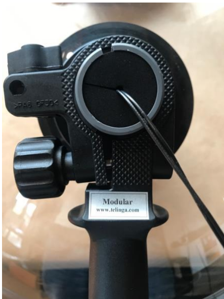
E. Cabling thru included Neoprene Stopper.
